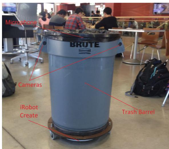
**Fig. 8** A standard Rubbermaid Brute trash barrel is mounted atop an iRobot Create platform. A laptop computer, hidden within the trash barrel, handles video and control commands
