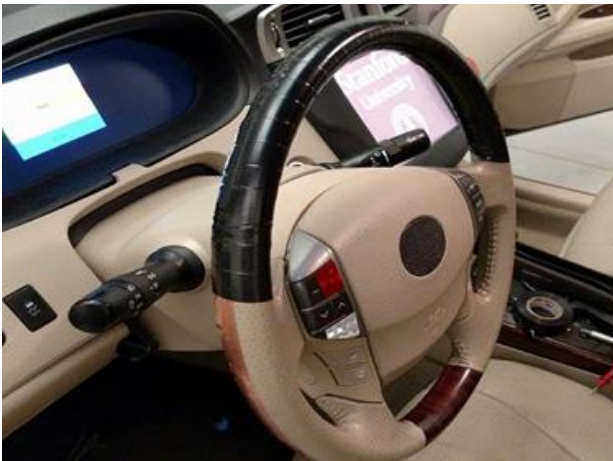
Figure 3: Simulator's steering wheel. Buttons used for takeover and copper tape used for influence.
