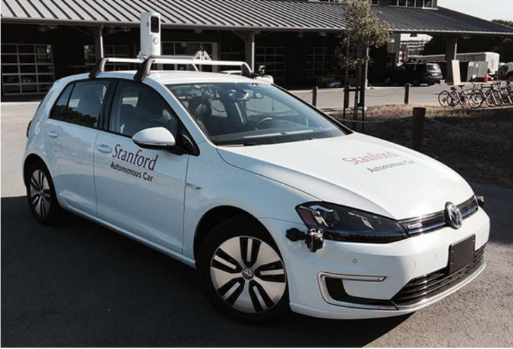
**Fig. 7** The Ghost Driver car features autonomous vehicle props like a laser-based detector, radar units, interior and exterior cameras and decals on the hood and doors
